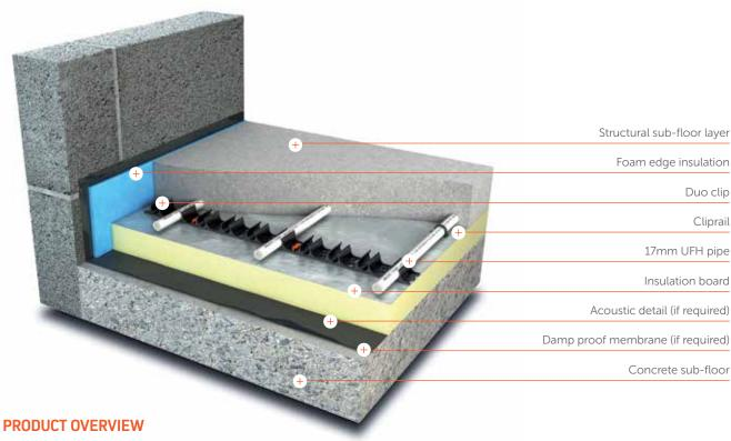
The AmbiDuoClip is a cost effective, hybrid solution that can be used where AmbiTak is the preferred option but the insulation board is either not deep enough to allow the pipe to be securely held with tacker clips alone or where the insulation is a PUR type board which lacks the required density to hold the clips in place.
