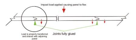
To achieve this, it is important to place a generous bead of adhesive to both faces of the T+G joint and then spread it using a brush. When the T+G edges are fully glued, you can see that an impact load applied to one panel is shared with
