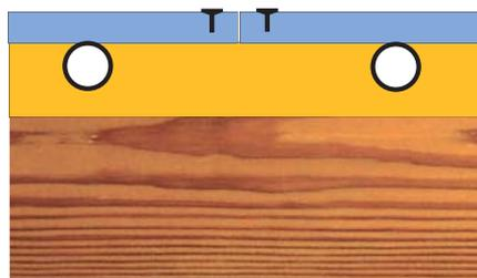
**(Above)** Overlay joints should be in the centre link between the grooves in the routed Ambi panels.
