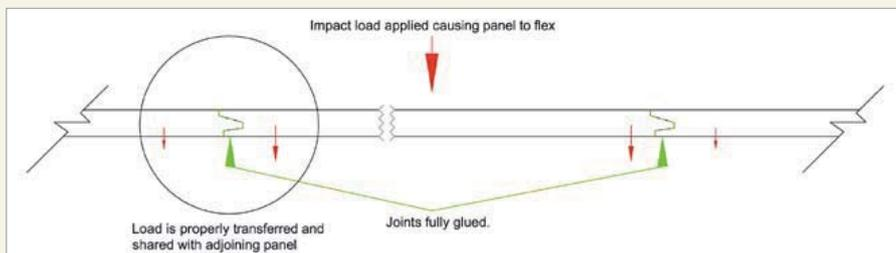
To achieve this, it is important to place a generous bead of adhesive to both faces of the T+G joint and then spread it using a brush. When the T+G edges are fully glued, you can see that an impact load applied to one panel is shared with the adjoining panels.
