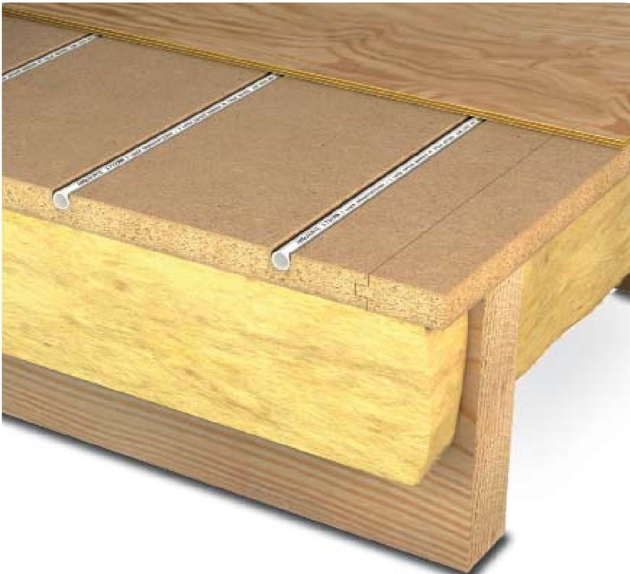
Ambichipboard | 22 System is designed specifically for turning a standard joisted floor into an underfloor heating system. Panels are pre-routed to accept 12mm UHF pipe. They are strong, moisture resistant and can be used and handled in exactly the same way as conventional chipboard panels.
